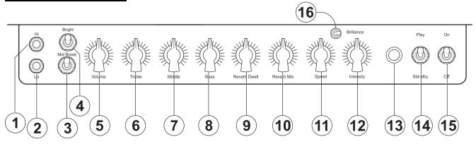
1. *Input - Hi:* This is the high impedance input for musical instruments. Use the Hi Input for the highest gain.
