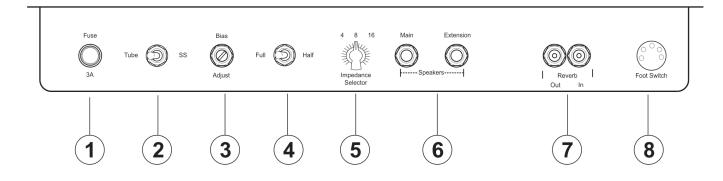
1. Fuse: Mains fuse for your amplifier. Replace only with the value stamped on the rear panel. Failure to comply with the recommended value could seriously damage the unit. Repeated fuse failures indicate a series electrical fault with the amplifier and should be addressed by a qualified service technician.
